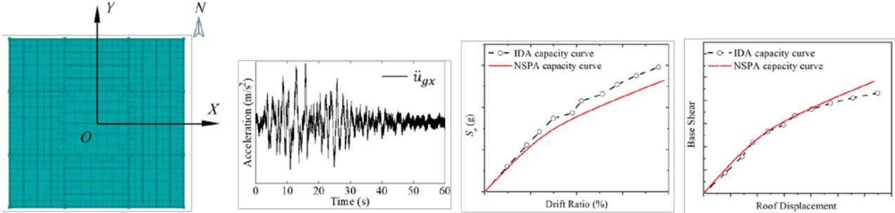
Figure 1. Footprint of a symmetric structure and schematic representation of capacity curve for unidirectional ground motions (the capacity curve is expressed in terms of SA versus drift ratio or Base shear versus roof displacement).
