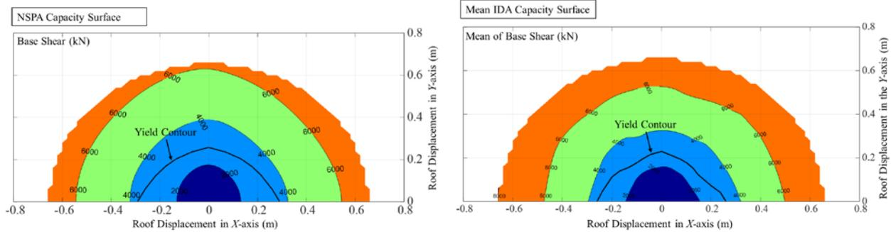
Figure 5. Capacity surface obtained by using the nonlinear static pushover analysis and the nonlinear incremental dynamic analysis.
